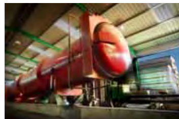
At 17m long and 3m diameter the new treatment vessel is capable of treating over 40m 3 in one charge.
